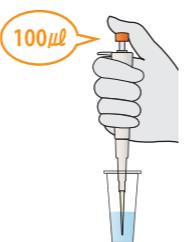
3. Add the mixed sample (100  $\mu$ L) into the sample hole of the test device using the 100  $\mu$ L pipette and press the [START] to initiate testing.
