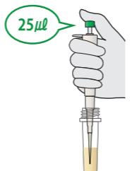
2. Use a 100  $\mu$ L pipette to mix the sample with diluent by pipetting, for 5~6 times.
