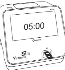
\* Strictly follow the test procedure including the amount of sample (25  $\mu$ L) used and the test time (5 min), as failure to do so may adversely affect test performance and/or produce invalid results.
