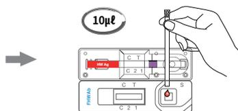
**3** Add 10µl of the serum, plasma or whole blood to the sample hole by using capillary tube
