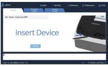
The Analyzer checks the conditions of inserted test device. If the test device has already been used, an E-1 error pops up.
