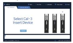
④ After inserting all the calibration devices, the analyzers performs the calibration analysis.
