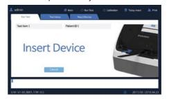
③ Analyzer checks the conditions of the inserted test device. If the test device has already been used, E-1 error pops up.
