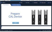
① Insert the Cal-1 Device into the test slot of the Analyzer.
