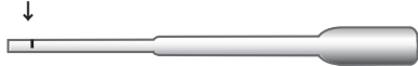
Figure1. A black line on the capillary tube is the indicator line for 10 \mu l.
