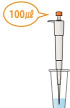
2. Add the mixed sample(100 µl) into the sample hole of the test device. Then, press the "Start" button.
