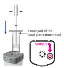
3 Place the stool pretreatment tool into the sample hole of the cartridge. And inject the sample into the tool.
